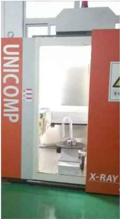
Unicomp X-Ray Inspect Bicycle Front Fork (made of aluminum/magnesium casting parts)
