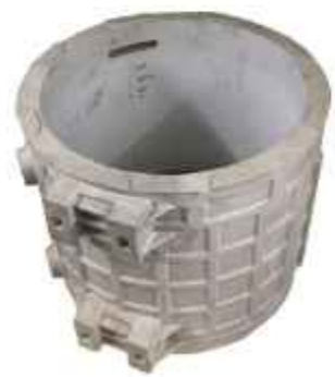
Battery Motor Housing (loose, slag)
