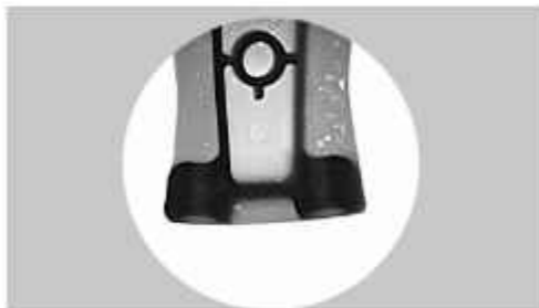
Aluminum casting pipe (shrinkage)
