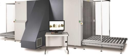
With a 1,500 mm (59.1 inches) wide x 1,650 mm (65.0 inches) high tunnel opening and a heavy-duty roller conveyor, the **Rapiscan 632XR** is designed to inspect pallets and other large cargo weighing up to 3,000 Kgs (6,600 pounds), and provide a horizontal view of the pallet. An optional belt conveyor is also available.
